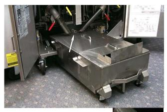
The filter pan slides under the fryer (above), connecting with a slip fitting (right). The slip fitting is located between the drain tubes (above, arrow).
